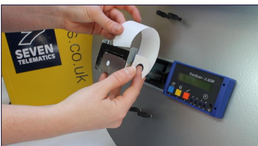
*Feed the leading edge of the paper into the slot at the top of the printer mechanism (press the blue button to operate the printer).*
