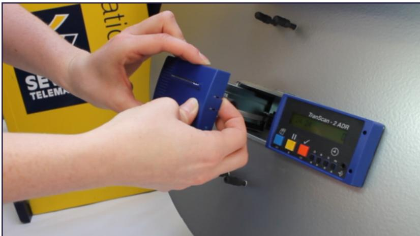
*To release the tray press the cover, pull out the tray and remove the cover by releasing the lip.*
