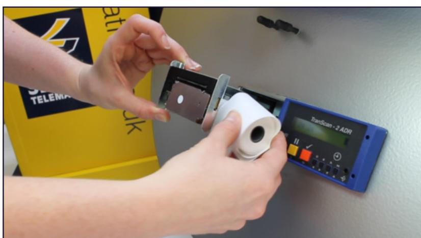
*Load the new paper roll onto the holder (the paper must feed forward from the top).*
