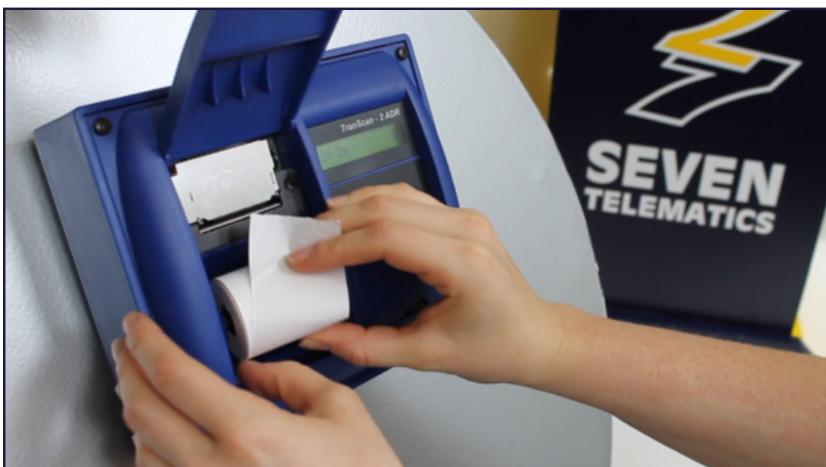
*Load the new paper roll onto the holder and fit it so that the paper feeds forward from the top of the roll.*
