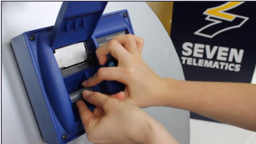
*Open the cover to remove the remains of the old paper roll (do not pull paper backwards through the printer as this may cause damage to the mechanism).*
