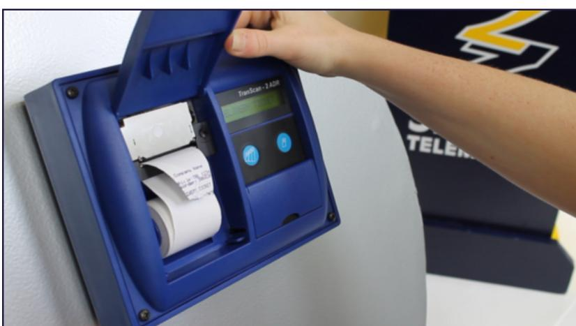
*Press either of the blue print buttons ( or ) to operate the printer.*
