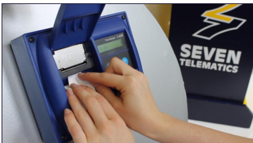
*Feed the leading edge of the paper into the slot at the bottom of the printer mechanism (if necessary cut the paper at an angle to ease feeding).*
