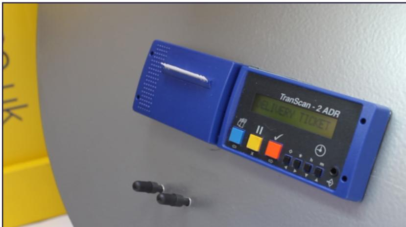
Press the button once and the display will read "DELIVERY TICKET", after a short pause a Delivery Ticket will be printed.
