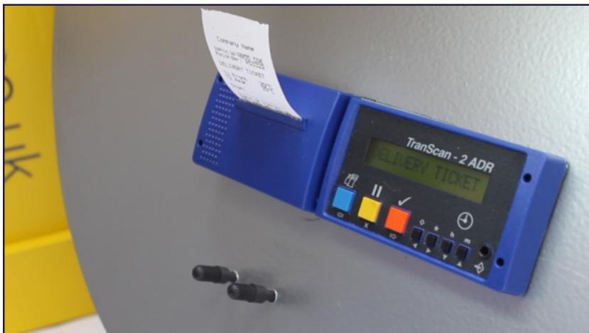
To abandon the printing of a DeliveryTicket, press the button and the display will read "abandoned".
